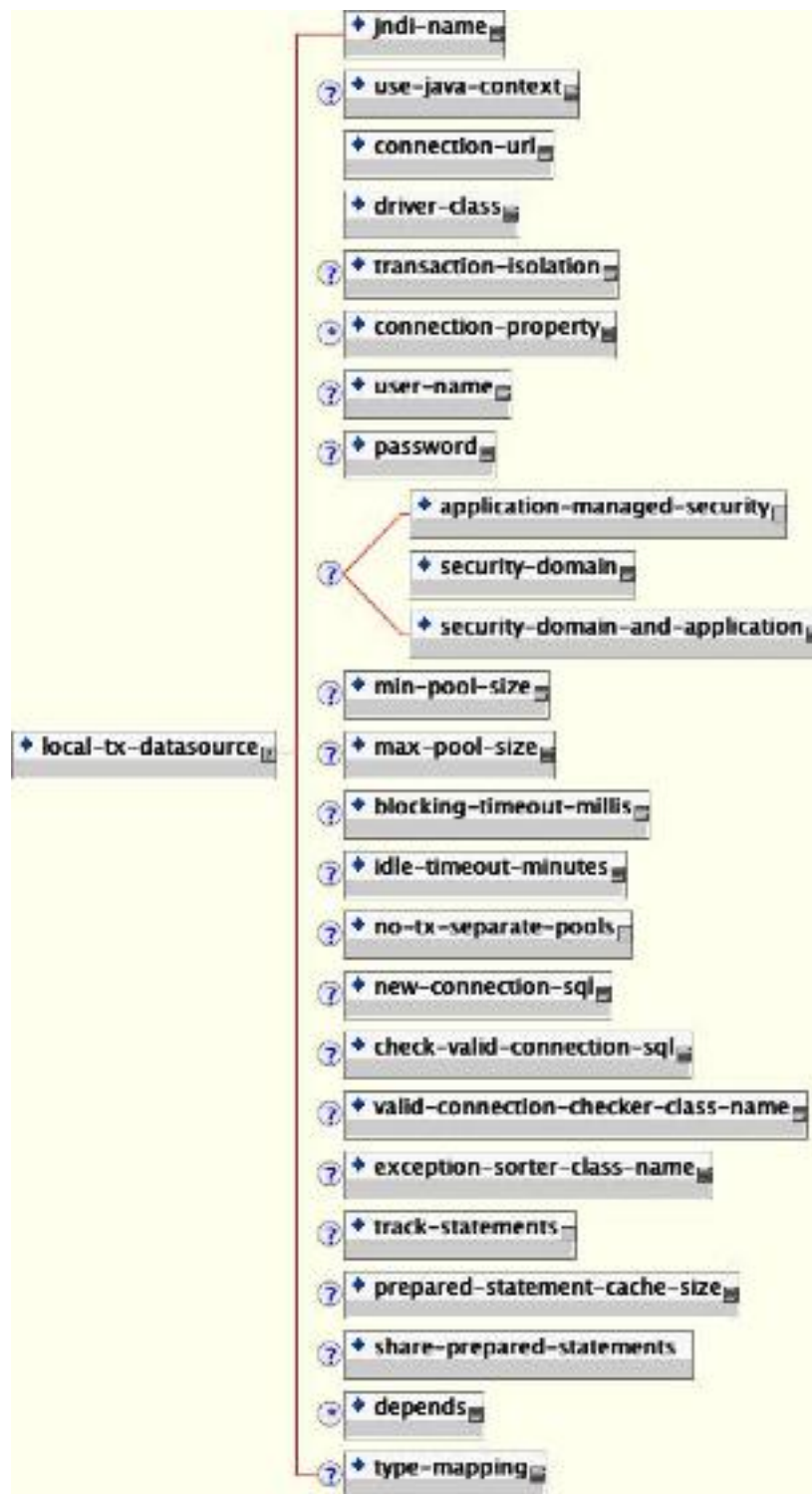
Figure 2.3. The non-XA DataSource configuration schema
