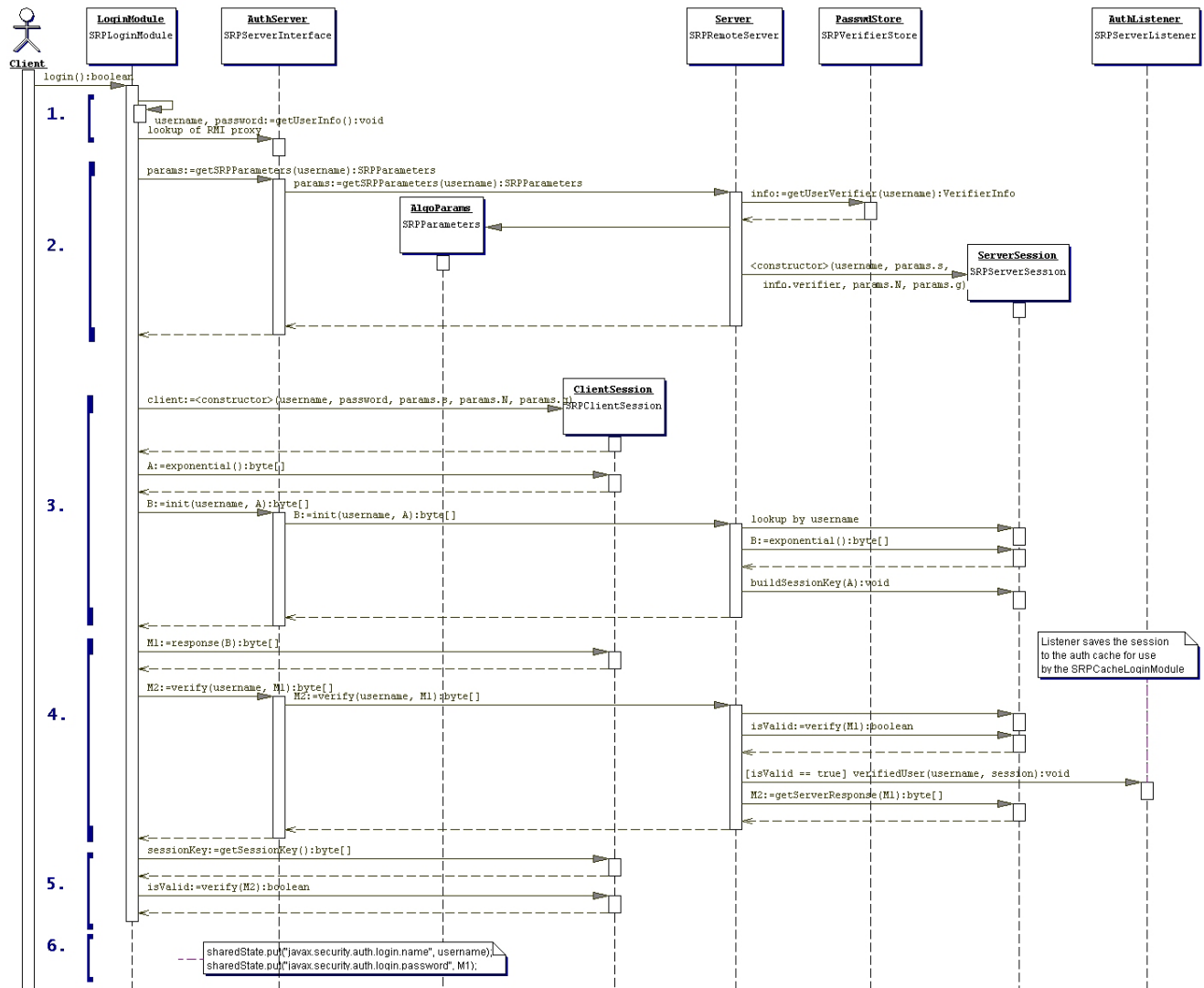
Figure 8-10, The SRP client-server authentication algorithm sequence diagram.
