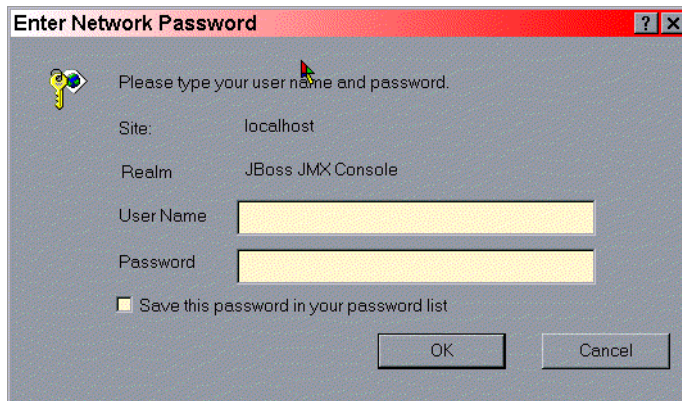
FIGURE 2-15. The jmx-console basic HTTP login dialog presented after making the changes shown in Listing 2-11.
