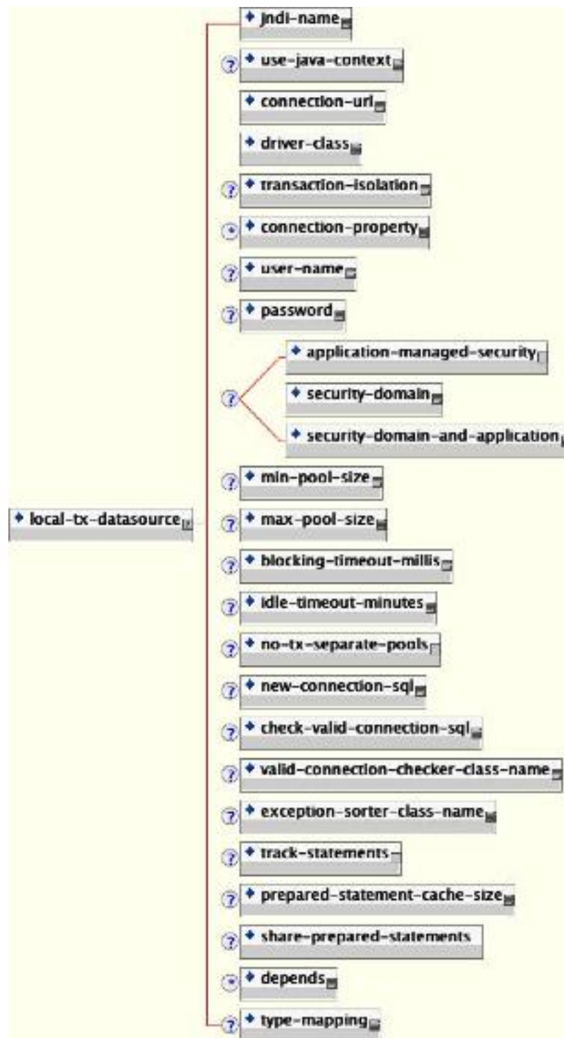
Figure 6.7. The non-XA DataSource configuration schema
