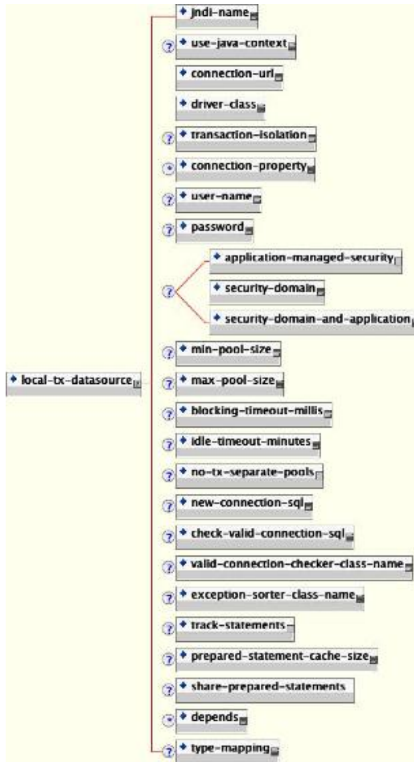
Figure 7.7. The non-XA DataSource configuration schema
