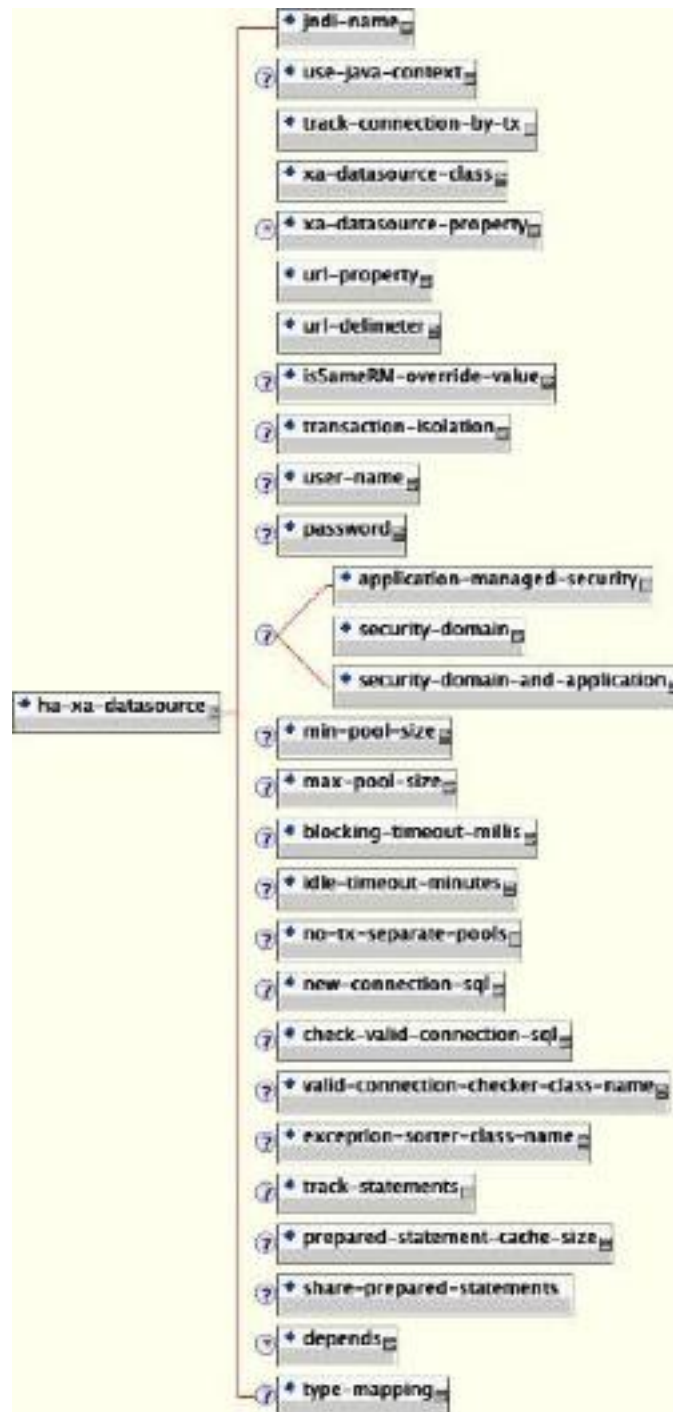
Figure 7.10. The schema for the experimental XA Datasource with failover
