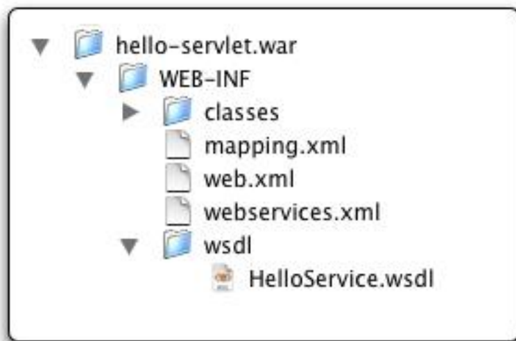
Figure 12.1. The structure of hello-servlet.war
