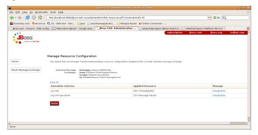
In order to allow the *SmooksTransformer* JBoss ESB ActionProcessor to leverage these configurations, simply make sure the *smooks-cdr.lst* file (in the root of the classpath) contains a list entry of http://<host>:<port>/jboss-esb-console/transform/smooks-config.jsp. where host and port refer to the address of the running Admin Conosle application.
