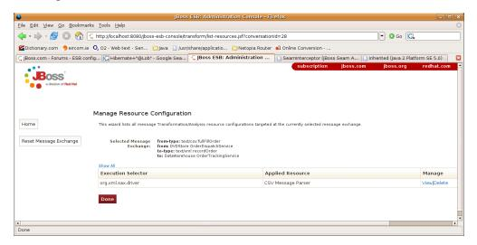
Next we need to create the XSLT configuration and target it at the same Message Exchange. Note that when this resource is applied by Smooks, the CSV message will be in a W3C DOM. The XML representation of this DOM will be of the following form (see <a href="Smooks CSVParser Docs">Smooks CSVParser Docs</a>):
