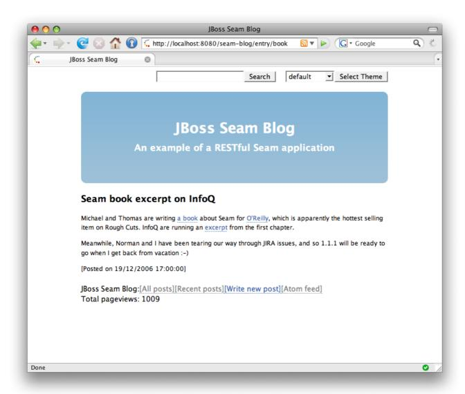
The Blog example demonstrates the use of "pull"-style MVC, where instead of using action listener methods to retrieve data and prepare the data for the view, the view pulls data from components as it is being rendered.
