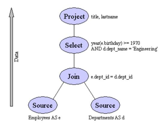
Data flows from the tables at the bottom upwards through the join, through the select, and finally through the project to produce the final results. The data passed between each node is logically a result set with columns and rows.
