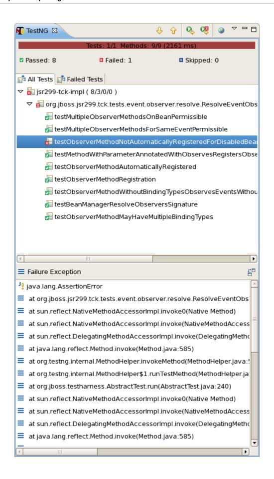
The view offers two lists. The first is a list of all methods (tests) in the class flagged as either passed or failed. The second is a list of methods (tests) in the class that failed. If there is a test failure, you can click on the method name to get the stacktrace leading up to the failure to display in the lower frame.
