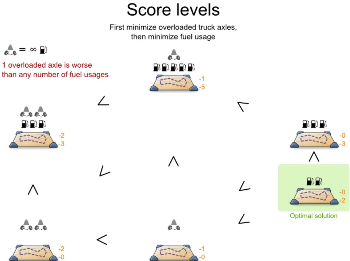
Score levels often employ score weighting per level. In such case, the hard constraint level usually makes the solution feasible and the soft constraint level maximizes profit by weighting the constraints on price.
