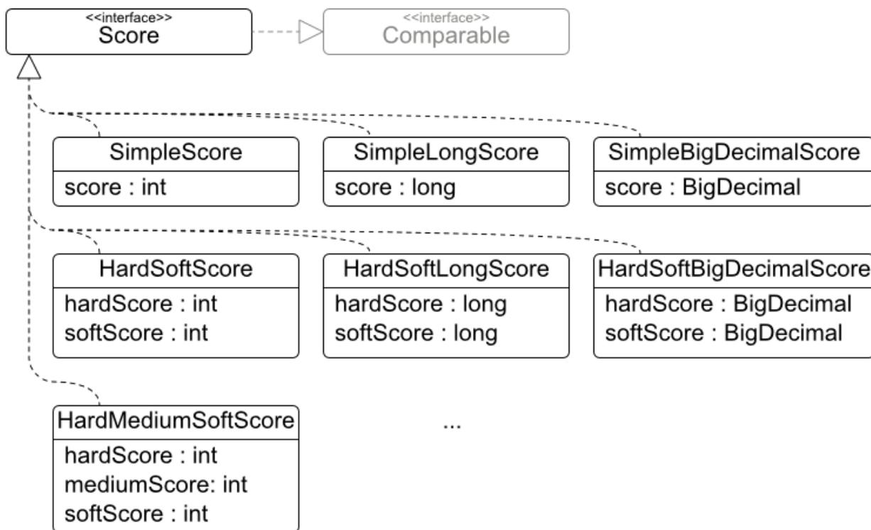
The `Score` implementation (for example `HardSoftScore`) must be the same throughout a `Solver` runtime. The `Score` implementation is configured in the solver configuration as a `ScoreDefinition`:
