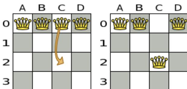
The new solution is called a *neighbor* of the original solution, because it can be reached in a single Move. Although a single move can change multiple queens, the neighbors of a solution should always be a very small subset of all possible solutions. For example, on that original solution, these are all possible changeMove's:
