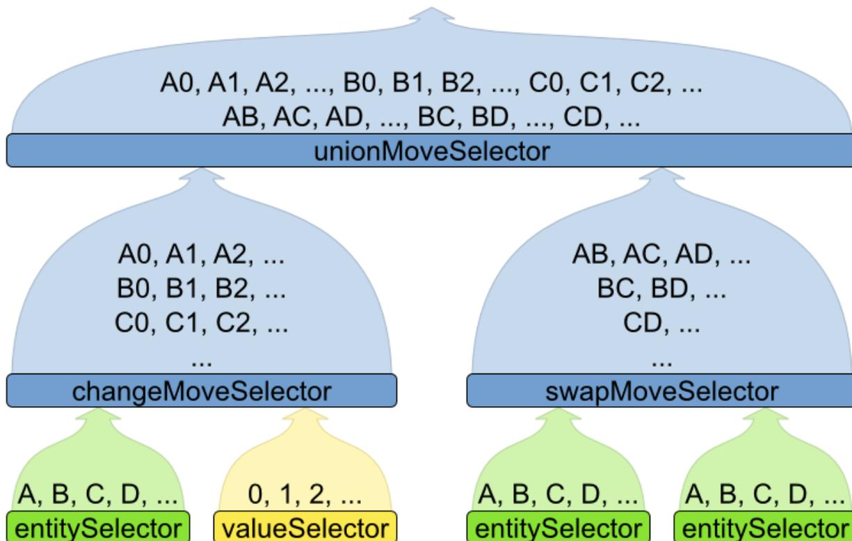
The root of this tree is a `MoveSelector` which is injected into the optimization algorithm implementation to be (partially) iterated in every step.
