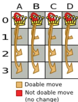
If we ignore the 4 changeMove's that have not impact and are therefore not doable, we can see that number of moves is  $n * (n - 1) = 12$ . This is far less than the number of possible solutions, which is  $n ^ n = 256$ . As the problem scales out, the number of possible moves increases far less than the number of possible solutions.
