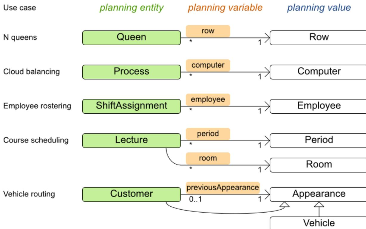
When in doubt, it's usually the many side of a many to one relationship that is the planning entity. For example in employee rostering, the planning entity class is `ShiftAssignment`, not `Employee`. Vehicle routing is special, because it uses a *chained planning variable*.
