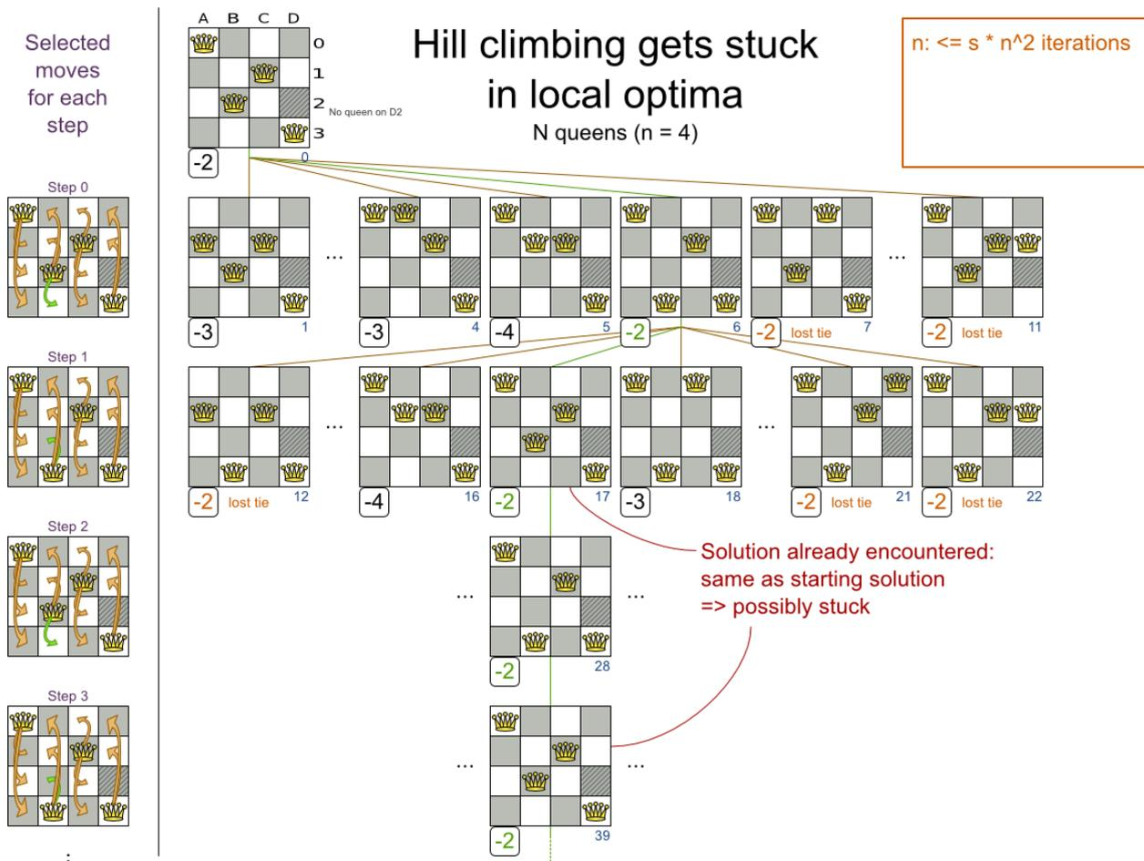
Improvements upon hill climbing (such as tabu search and simulated annealing) address the problem of being stuck in local optima.
