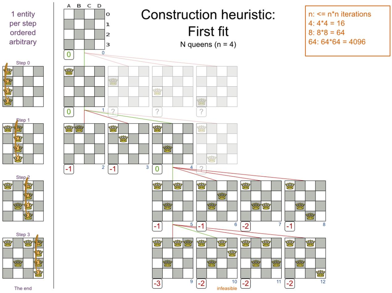
Notice that it starts with putting `Queen A` into row 0 (and never moving it later), which makes it impossible to reach the optimal solution. Suffixing this construction heuristic with metaheuristics can remedy that.
