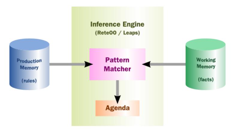
Figure 1.1. High-level View of a Production Rule System
