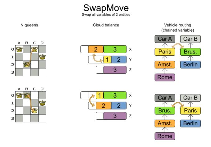
Although a SwapMove on a single variable is essentially just 2 ChangeMoves, it's often the winning step where the first of the 2 ChangeMoves would not be the winning step because it leave the solution in a state with broken hard constraints. For example: swapping the room of 2 lectures
