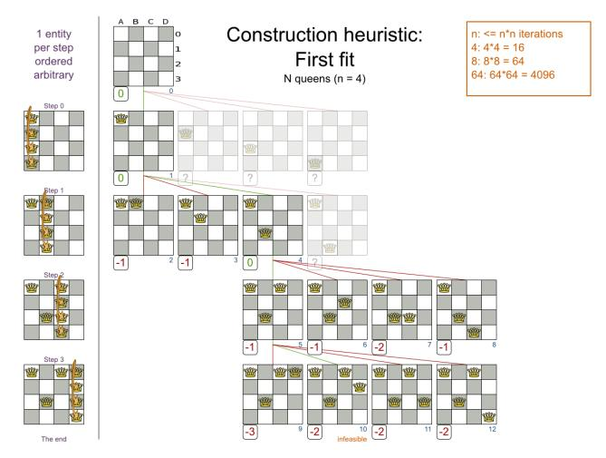
Notice that it starts with putting <code>Queen</code> A into row 0 (and never moving it later), which makes it impossible to reach the optimal solution. Suffixing this construction heuristic with metaheuristics can remedy that.
