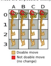
If we ignore the 4 <code>changeMove</code>'s that have not impact and are therefore not doable, we can see that number of moves is n \* (n - 1) = 12. This is far less than the number of possible solutions, which is n \* n = 256. As the problem scales out, the number of possible moves increases far less than the number of possible solutions.
