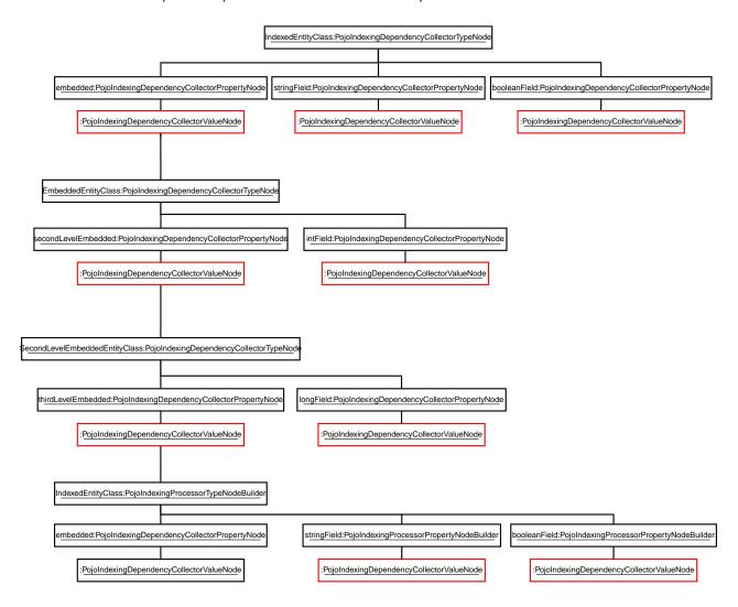
The value nodes in red are those that we will mark as a dependency using PojoIndexingDependencyCollectorValueNode#collectDependency. The embedded property at the bottom will be detected as not being used during indexing, so the corresponding value node will not be marked as a dependency, but all the other value nodes will.
