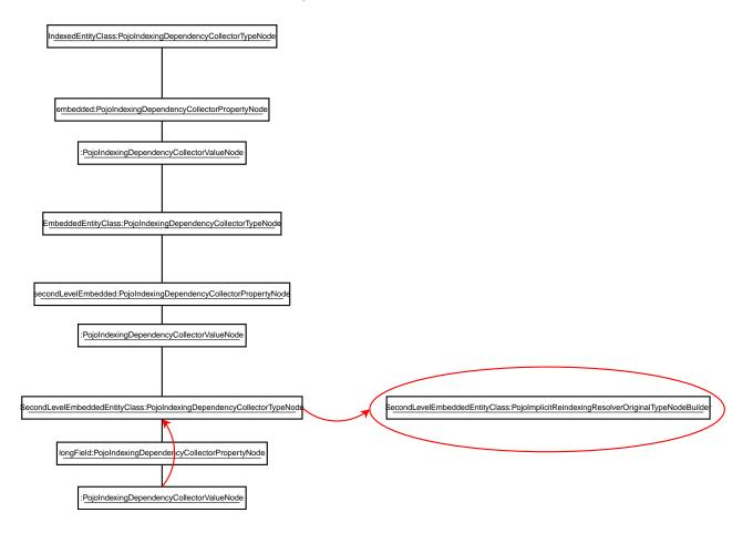
From there, the reindexing resolver builder is passed to the next dependency collector value node using the PojoIndexingDependencyCollectorValueNode#markForReindexing method. This method also takes as a parameter the path to the property that is depended on, in this case longField.
