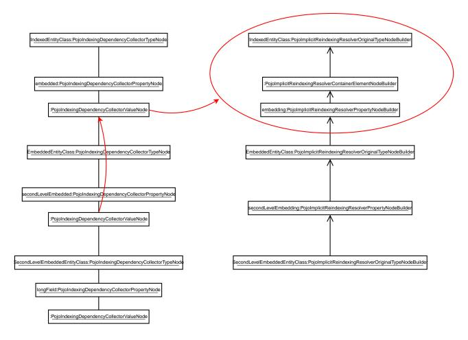
Once we reach the dependency collector root, we are almost done. The reindexing resolver builder tree has been populated with every node needed to reindex IndexedEntityClass whenever a change occurs in the longField property of SecondLevelEmbeddedEntityClass.
