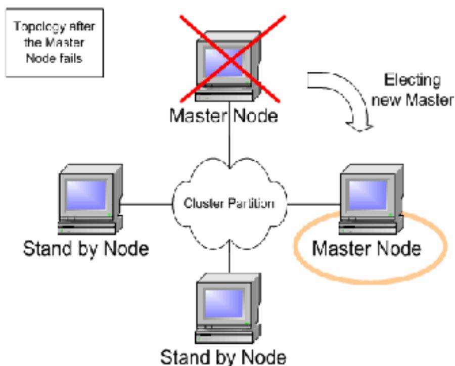
**Figure 4.1. Topology after the Master Node fails**
