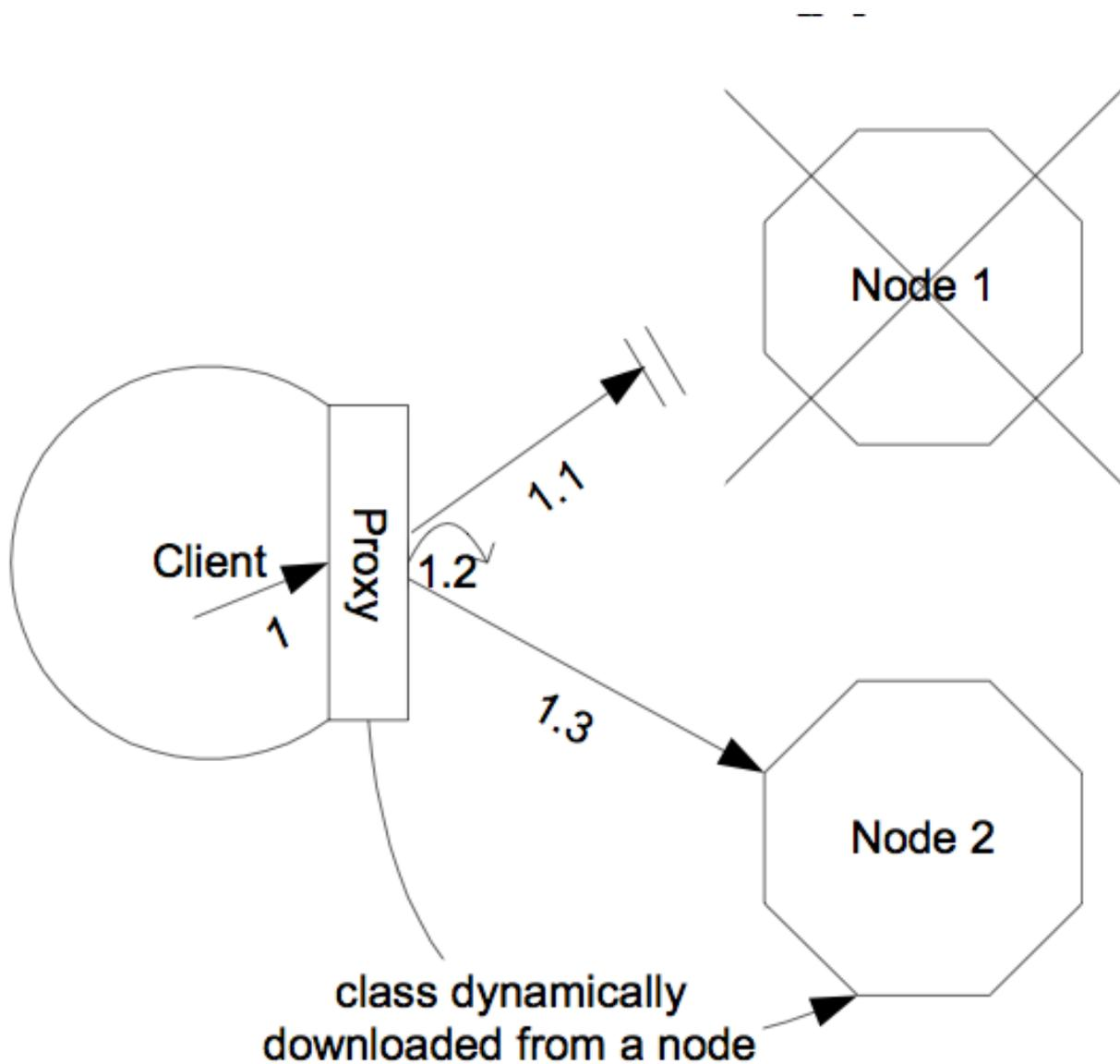
**Figure 2.2. The client-side interceptor (proxy) architecture for clustering**
