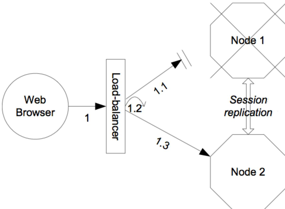
**Figure 2.3. The external load balancer architecture for clustering**
