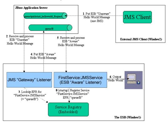
After starting the ESB in Window1 and before any "Hello World" messages are put on the bus, the "FirstService:SimpleJMSService" Service is registered with the Registry Service.
