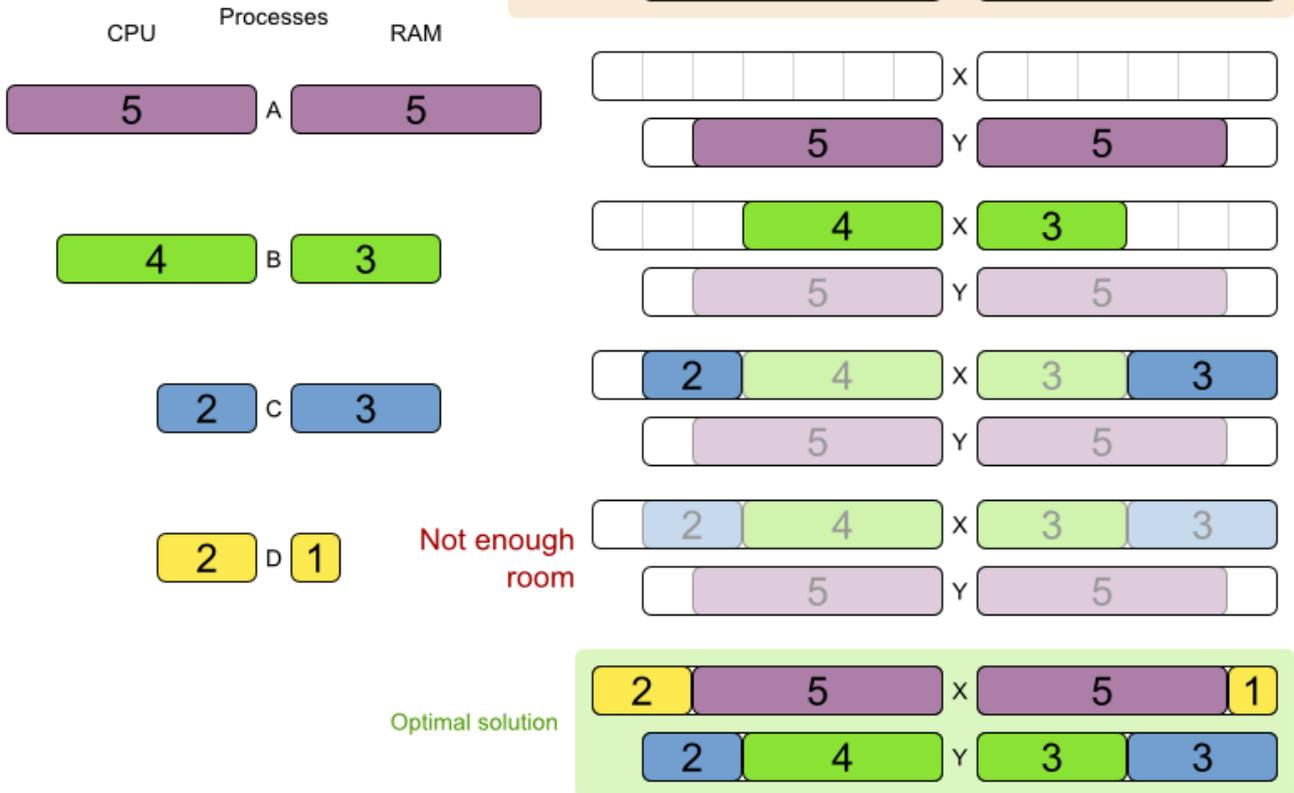
The simple algorithm used here is the *First Fit Decreasing* algorithm, which assigns the bigger processes first and assigns the smaller processes to the remaining space. As you can see, it is not optimal, as it does not leave enough room to assign the yellow process D.
