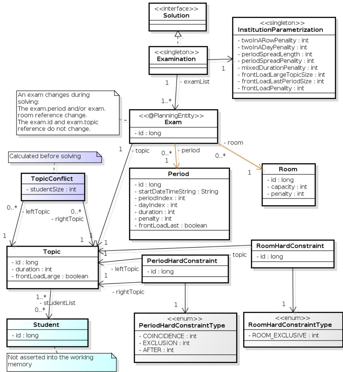
Figure 3. Examination Domain Class Diagram
