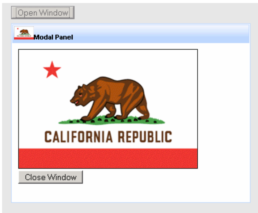
Figure 6.74. The <rich:modalPanel> is opened in "closest" to an observer layer. Other layers are dimmed by blocking <div> (gray on the picture).
