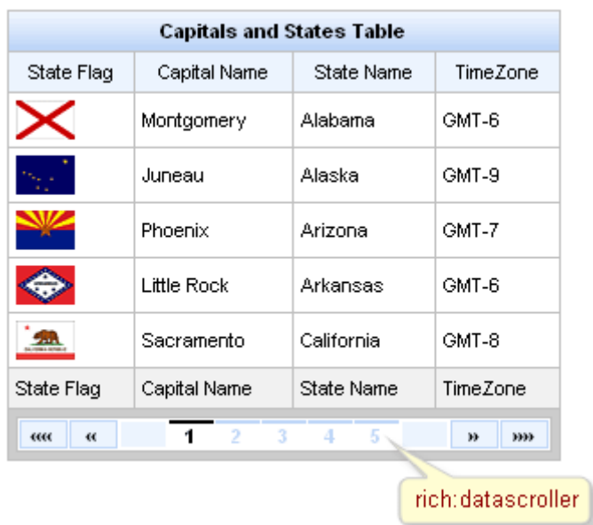
Figure 10.17. The <rich:dataScroller> component
