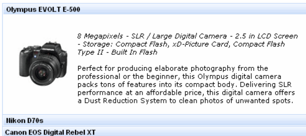
Figure 9.3. A <rich:accordion> component containing three <rich:accordionItem> components
