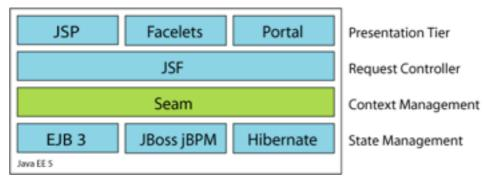
It turns out that the combination of Seam, JSF and EJB3 is *the* simplest way to write a complex web application in Java. You won't believe how little code is required!
