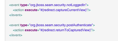
Note that login redirection is implemented as a conversation-scoped mechanism, so don't end the conversation in your authenticate() method.
