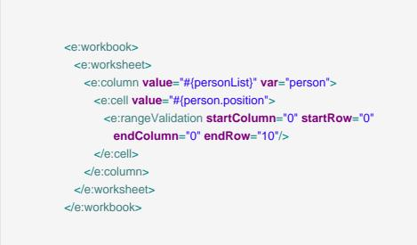
adds validation to a cell specifying that the value must be in the values specified in range A1:A10.
