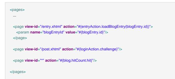
Notice that the example is using page actions for some other functionality—the login challenge, and the pageview counter. Also notice the use of a parameter in the page action method binding. This is not a standard feature of JSF EL, but Seam lets you use it, not just for page actions, but also in JSF method bindings.
