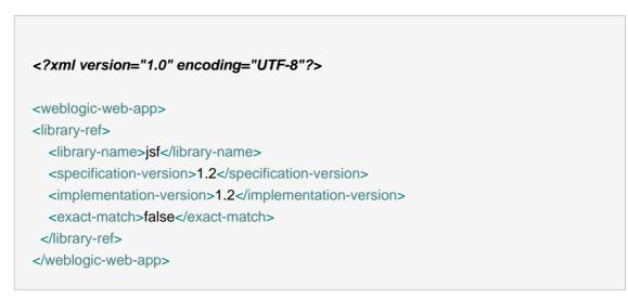
• This file and the element library-ref tells Weblogic that this application will using the deployed JSF libraries. This is needed in both this file and the weblogic-application.xml file because both applications require access.
