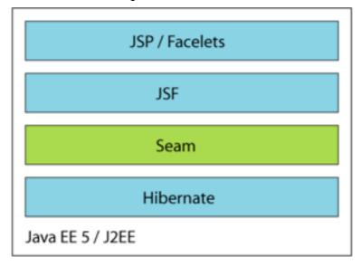
Seam JavaBean components do not provide declarative transaction demarcation like session beans do. You *could* manage your transactions manually using the JTA <code>UserTransaction</code> or declaratively using Seam's <code>@Transactional</code> annotation. But most applications will just use Seam managed transactions when using Hibernate with JavaBeans.
