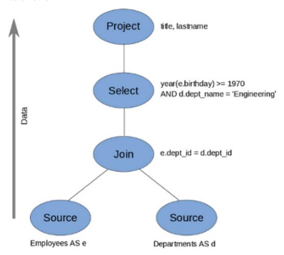
Data flows from the tables at the bottom upwards through the join, through the select, and finally through the project to produce the final results. The data passed between each node is logically a result set with columns and rows.
