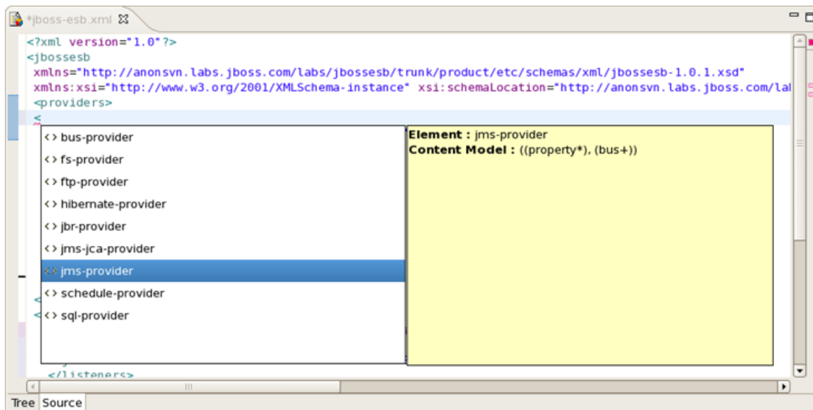
Figure 3.17. Content Assist for ESB XML file
