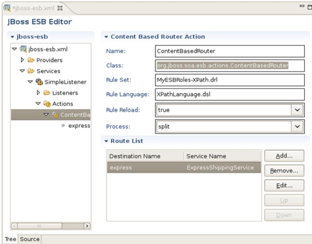
**Figure 3.10. Form Editor for Content Based Router**
